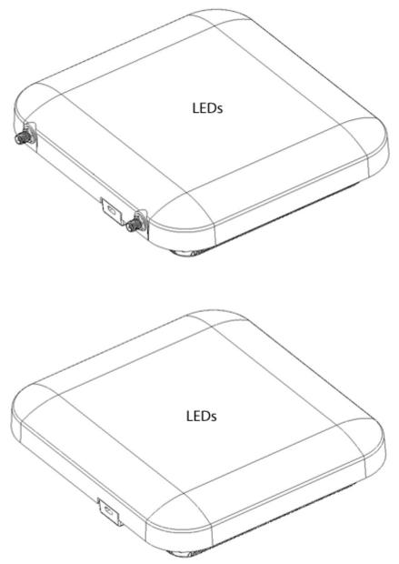
The LEDs provide a status display indicating error conditions, transmission, and network activity for the 5 GHz 802.11ac (amber) radio and the 2.4 GHz 802.11n (green) radio.
