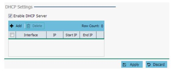
20. Select **Enable DHCP Server** to ensure the Access Point can provision IP addresses to requesting clients over the specified interface.
